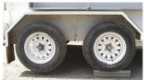
Non-load sharing suspension with no wheel travel and similar ride to a box trailer.
